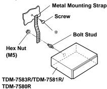
3 Slide the TDM-7583R/TDM-7581R/TDM-7580R into the dashboard. When the unit is in place, make sure the locking pins are fully seated in the down position. This can be done by pressing firmly in on the unit while pushing the locking pin down with a small screwdriver. This ensures that the unit is properly locked and will not accidentally come out from the dashboard. Install the Detachable Front Panel.
